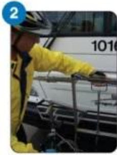
2. Squeeze handle and pull rack down.
