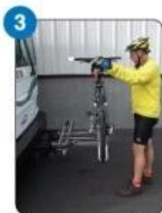
3 Lift bike into rack with front tire facing the support arm.
