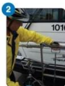
2 Squeeze handle and pull rack down.
