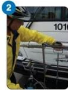
2 Squeeze handle and pull rack down.
