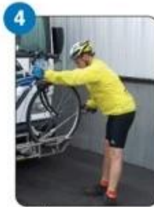
4 Pull support arm out, up, and over front tire.
