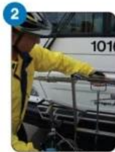
2 Squeeze handle and pull rack down.
